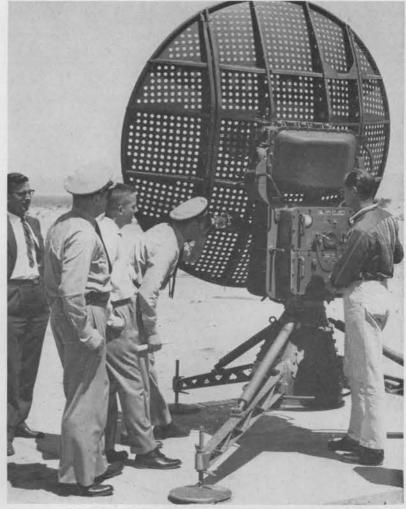
METEOROLOGISTS of the Inter-Range Instrumentation Group meeting at Salton Sea Test Base recently were given a tour of facilities. Here, members of the group examine a GMD upper air measurement system that records weather information from radios and balloons released into the atmosphere. At right is T. N. Earp.
